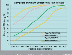
Values are Minimum Efficiency Reporting Values (MERV) when evaluated per ASHRAE Standard 52.2. The Camfil Farr Riga-Flo<sup>®</sup> PH provides high efficiency ASHRAE air filtration performance in a compact, supported media design. The materials of construction preclude contaminant amplification as all components are inert with respect to supporting the growth of captured bacteria or other viable contaminants. The Riga-Flo:
